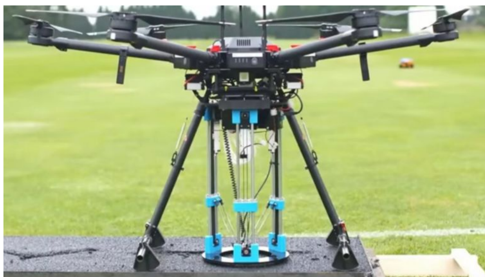
Figure 9: Road-repairing drone developed by academics at the University of Leeds
